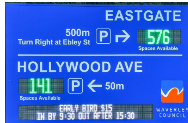
Figure 4.10: Variable Message signage
