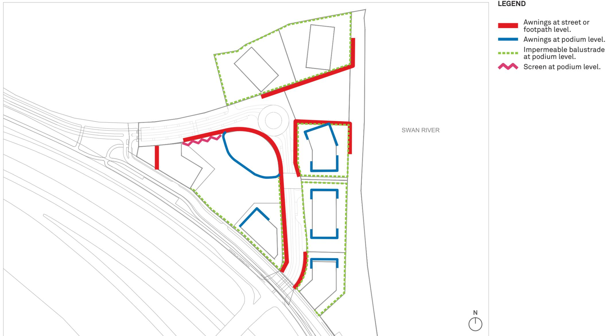
Figure 62: Design elements required to minimise wind impacts. The awnings identified in this drawing are required to mitigate wind impacts. Awnings are also required in other areas, as stipulated in the Site Specific Guidelines. Note: These design solutions are provided as guidance and alternative approaches may be approved where they are supported by a wind impact statement.
