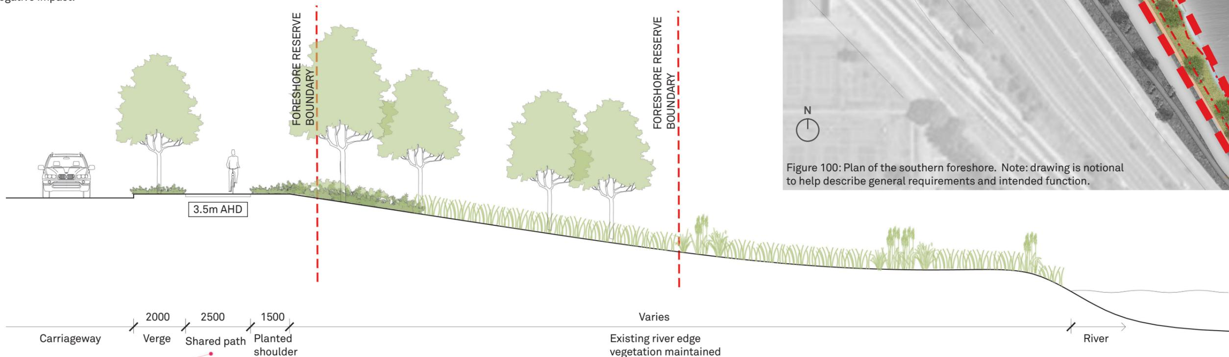
Figure 101: Section drawing of the southern foreshore in the area indicated. Note: drawing is notional to help describe general requirements and intended function.
