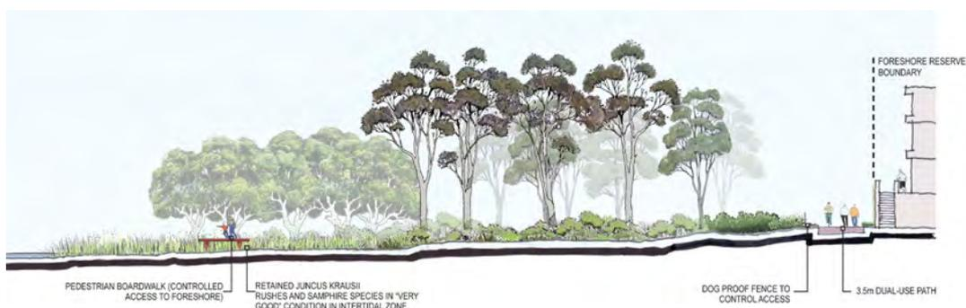
FIGURE 57: CONCEPT FOR AREAS OF NATIVE RIVERINE VEGETATION (NORTH EAST PART OF THE SITE) WITH APPROPRIATE MEASURES TAKEN SUCH AS CONSTRUCTION OF DOG FENCES TO PROTECT THE VEGETATIVE AREAS.
