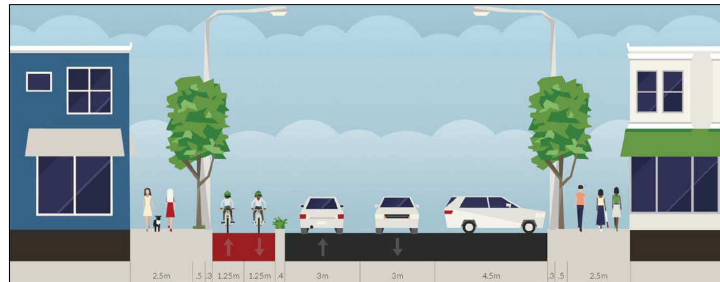
Figure 15-2: Potential Albany Highway cross section with bi-directional cycle lanes and angled parking
