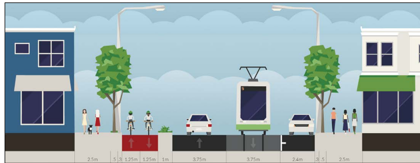
Figure 15-3: Potential Albany Highway cross section with bi-directional cycle lanes and shared light rail transit/general traffic lanes
