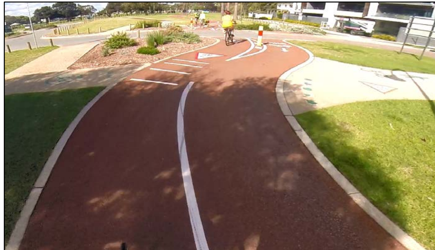
Figure 8-3: Lack of wayfinding at Sir James Mitchell Park foreshore path intersection with Coode Street path.
