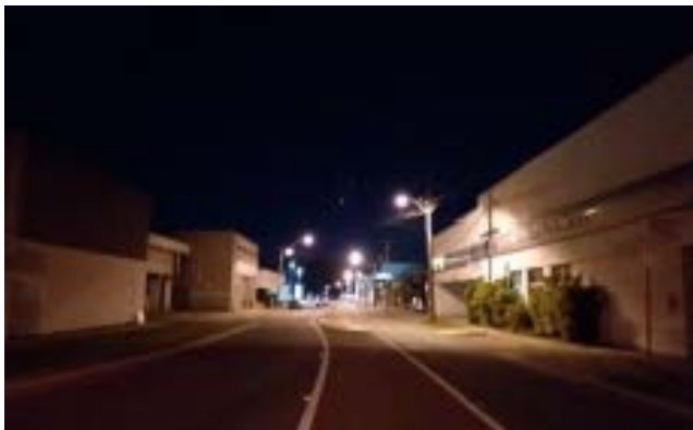
Low lighting levels, concentrated in sections, 4 lights not working
