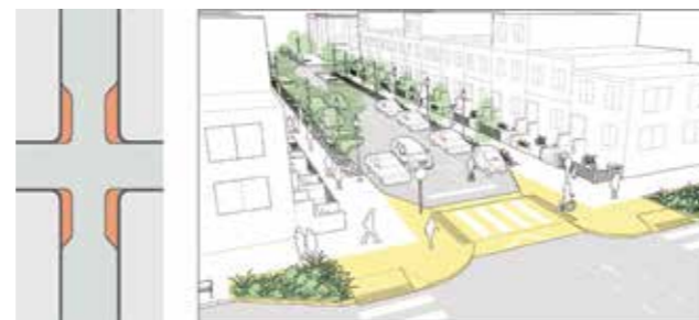
Narrowed street entrances
