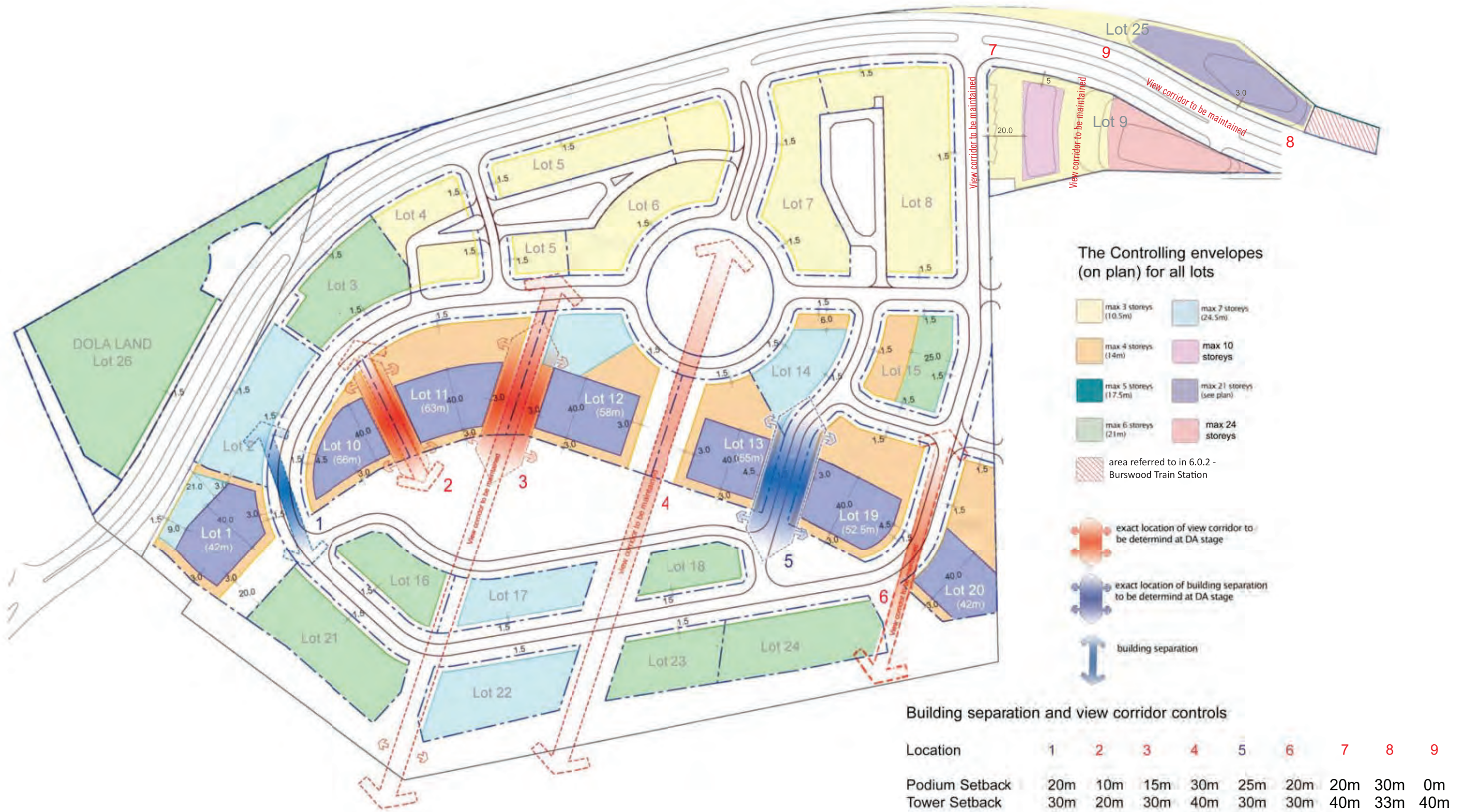
FIGURE 24: UPDATED BUILDING CONTROL ENVELOPES
