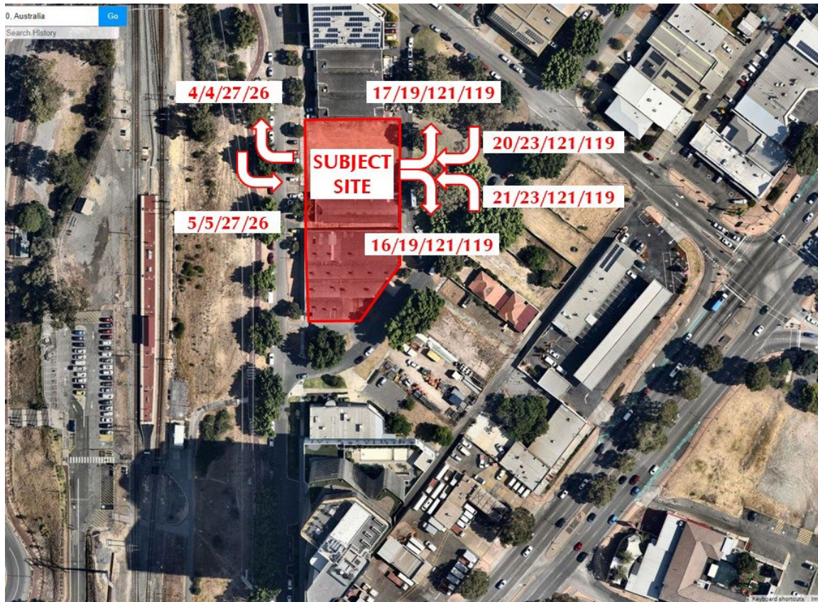
Figure 3. Estimated traffic movements for the proposed development – Friday peak hour/Sunday peak hour and Friday /Sunday total daily trips
