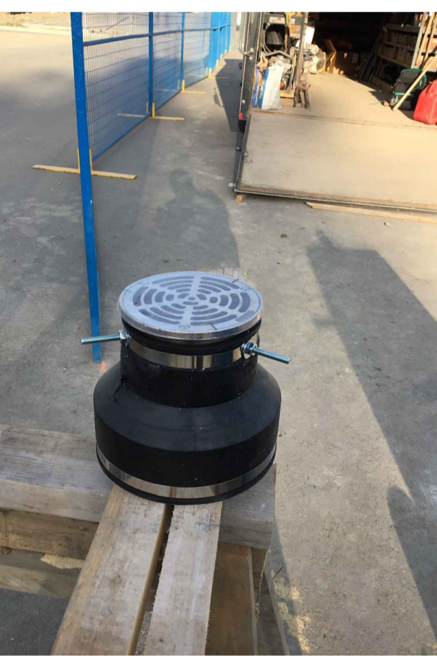
EXAMPLE OF MODIFIED AREA DRAIN SURROUND SO AS TO PREVENT SINKING BELOW FLUSH
