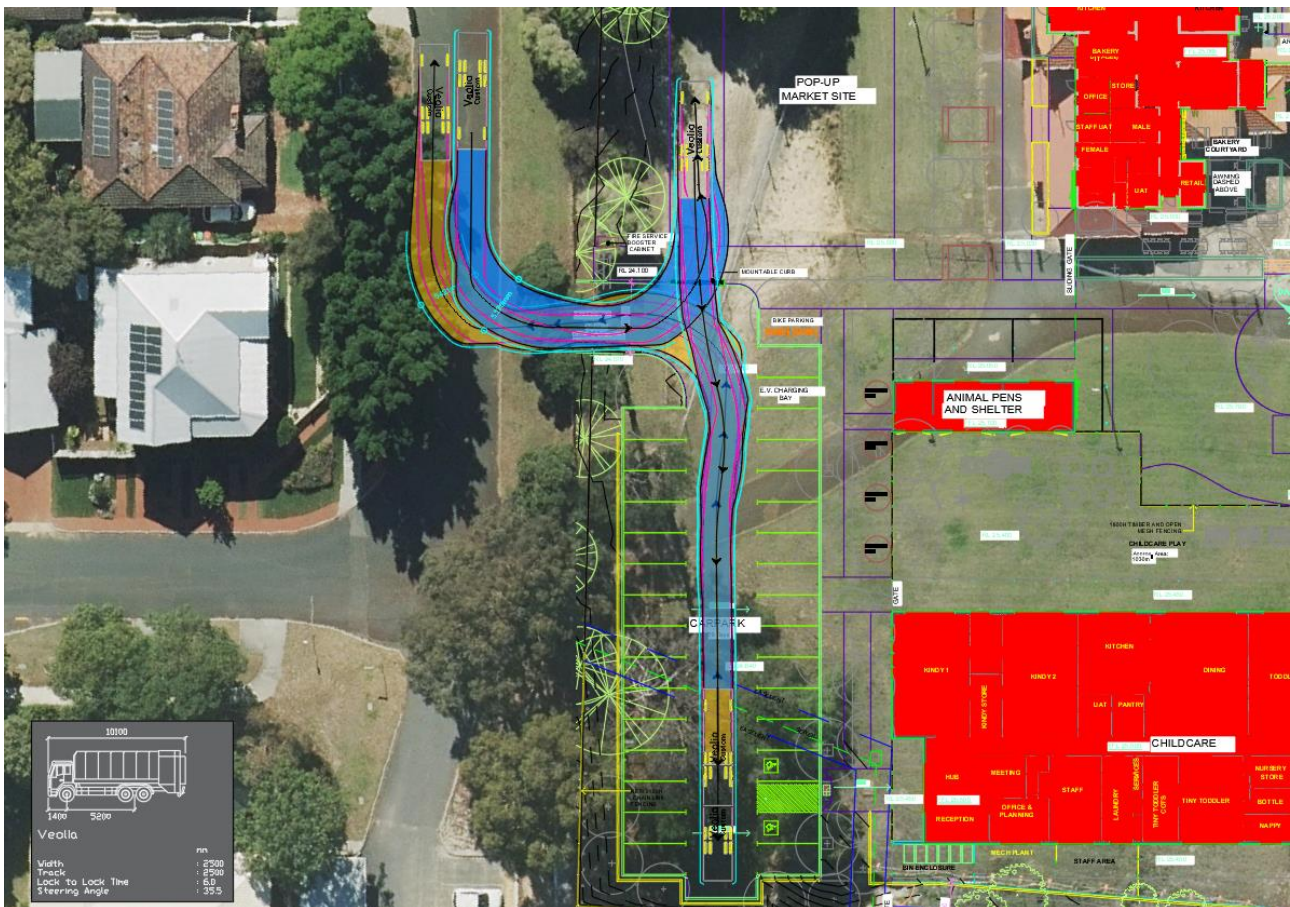
Figure 2-3 Swept Path – Waste Collection (Childcare Centre)
