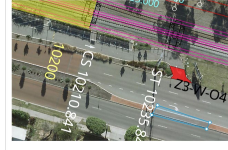
Ch 10250 Scope Remove and reinstate 120m2 and kerbing
