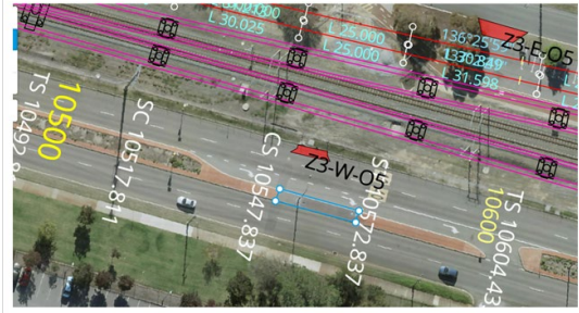
Ch 10550 Scope Remove and reinstate 120m2 and kerbing
