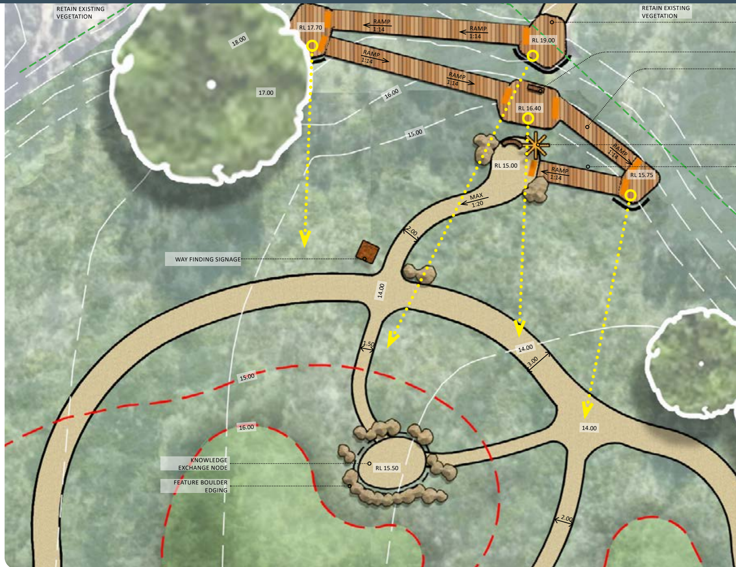
CLAY ROAD BASE OVERLAID WITH POLY SEALANT FOR ALL ABILITY ACCESS
